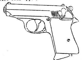
The blow-back type of auto is so-named because it is just that. As the gun is fired, the cartridge case starts rearwards at the same time as the bullet moves the other way, propelled by exactly the same impulse (Newton's Third Law, and all that), but is restrained by the mass of the breech-block and a strong recoil spring. In this way, the bullet leaves the gun before the case neck clears the breach, allowing pressure to drop to a safe level.
